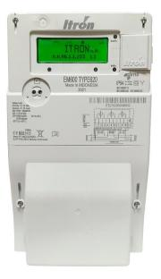
Itron EM620 is a static, polyphase, four-quadrant, multi-rate, smart meter. It is intended for commercial / industrial applications and suitable for Low Voltage / High Voltage Current Transformer connected operated networks (LVCT, HVCT), as well as low voltage Direct Connected operated network (LVDC).
