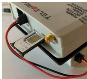
Kit GSM Telemetry Modem Teleorigin RB900SG
