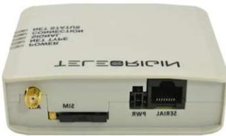
Teleorigin RB900SG - Modem GSM/GPRS/LTE/4G
